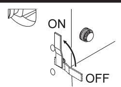
Figure 44. Water System ON/OFF Valve
